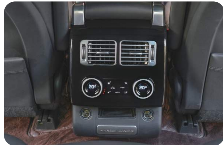
ZF-5011 后排空调控制面板 Rear seats climate control panel
